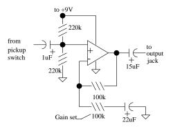
A preamp from a TL071 op amp. The gain set resistor lets you customize the gain. As shown, it is 2. Lowering the Gain Set resistor lets you raise the gain. You get distortion at high gains.
