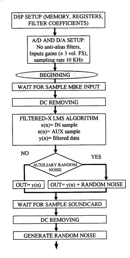
Figure 4. Programming structure of the active noise controller
