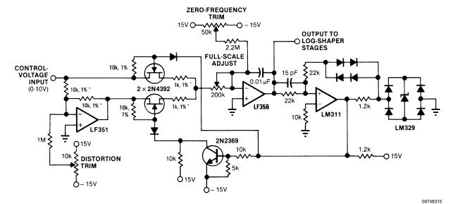
Adjust distortion for minimum at 1 Hz to 10 Hz Adjust full-scale for 30 kHz at 10V input All diodes = 1N4148
