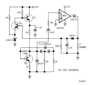
FIGURE 1. Phase-shift sine wave oscillators combine simplicity with versatility. This 12 kHz design can deliver 5 Vp-p to the  $8\Omega$  load with about 2% distortion.
