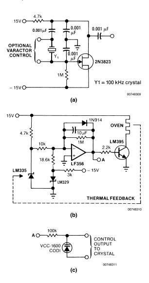
FIGURE 8. Stable quartz-crystal oscillators can operate with a single active device (a). You can achieve maximum frequency stability by mounting the oscillator in an oven and using a temperature-controlling circuit (b). A varactor network (c) can also accomplish crystal fine tuning. Here, the varactor replaces the oven and retunes the crystal by changing its load capacitances.
