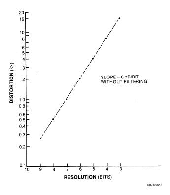
FIGURE 17. Distortion levels decrease with increasing digital word length. Although additional filtering can considerably improve the distortion levels (to 0.1% from 0.5% for the 8-bit case), you're better off using a long digital word.
