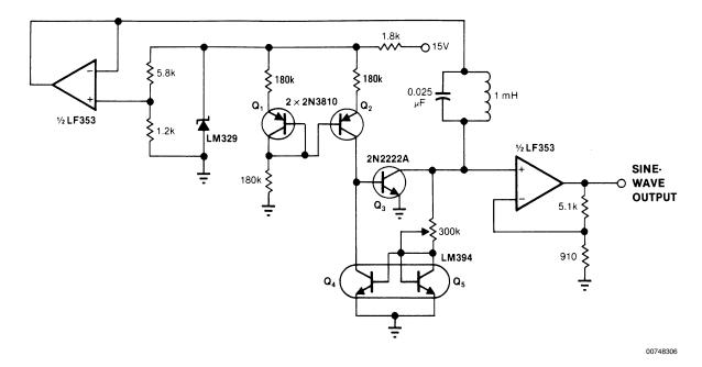
FIGURE 5. LC sine wave sources offer high stability and reasonable distortion levels. Transistors Q1 through Q5 implement a negative-resistance amplifier. The LM329, LF353 combination eliminates power-supply dependence.
