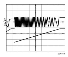
FIGURE 13. Rapid frequency sweeping is an inherent feature of *Figure 12's* voltage-controlled sine wave oscillator. You can sweep this VCO from 1 Hz to 30 kHz with a 10V input signal; the output settles quickly.
