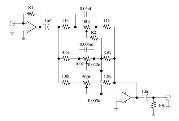
R1 is left up to the user depending on gain needs, R2 is unknown - experiment, the op-amps are not critical, any standard ones could be used. This circuit was originally intended for home audio use, but should be able to be hacked into an effect circuit with very minor modification.
